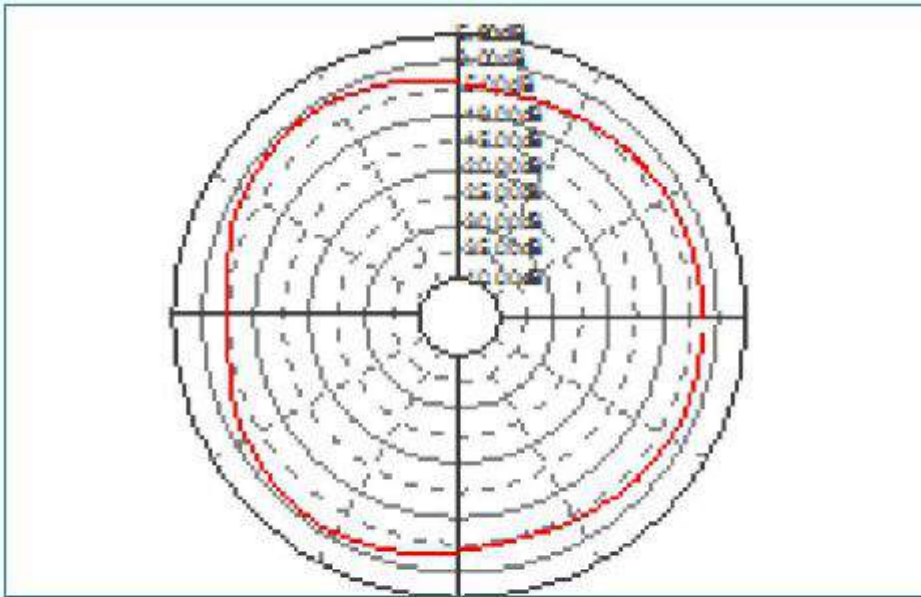
Typical Radiation Patterns for 1710-2170 MHz frequency band, on Reference Board 50x110mm for yx plane
